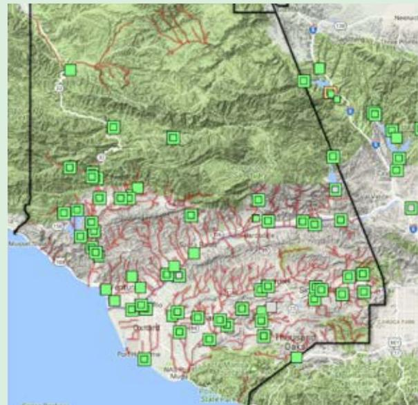
The rain gauges (+) are distributed throughout the county, including in the undeveloped forest areas to the north, in order to report rain in the watershed. The stream gauges (■) are located downstream on the larger rivers. The district monitors gauges outside the county in watersheds that drain into Ventura County.
